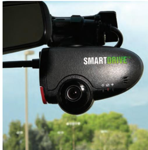
Last year, Access Services purchased the SmartDrive camera system for installation in all Access-owned vehicles. SmartDrive is a comprehensive on-board camera system that records events and then provides extensive information to Access and contractor staff, who, in turn, can coach drivers and ultimately correct unsafe driving behavior.
